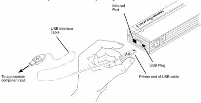
FIGURE 7. Connecting the PocketJet to your computer
